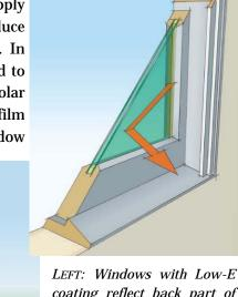
LEFT: Windows with Low-E coating reflect back part of the summer sun. ABOVE: Windows with Low-E coating reflect back part of room's heat. IMAGE SOURCE: Energy Savers, U.S. Department of Energy.
