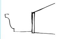
K-style gutters are appropriate for closed eaves and open eaves with a closed rafter. They are not appropriate when fascia board is not present.
