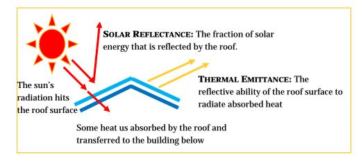
Cool roofs reflect and emits the sun's heat back into the sky instead of transferring it to the structure. Their average energy saving range from 7-10%. There are several different types of cool roofs. They range from coatings for metal roofs and flat roofs to reflective granules on asphalt and other synthetic shingles. \_\_\_\_\_\_
