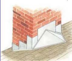
the most likely place for a leak. Metal z -flashing or step-flashing are recommended to ensure that there is no water intrusion. Often roofing cement is applied to the joint to create a water- tight juncture; however, the cement will eventually crack, thus allowing water in.
