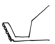
Built-in gutters are appropriate for open eaves and boxed eaves.
