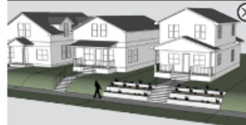
SLOPE TERRACED WITH RETAINING WALLS
