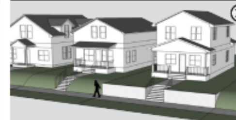
LOT LEVELED WITH A HIGH RETAINING WALL
