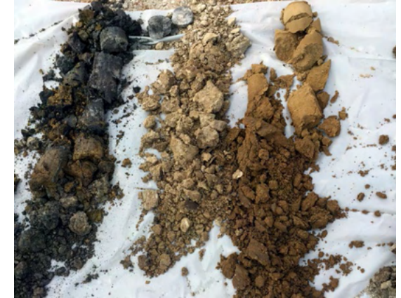
Subsurface soil sampling cores are collected to determine environmental impacts.
