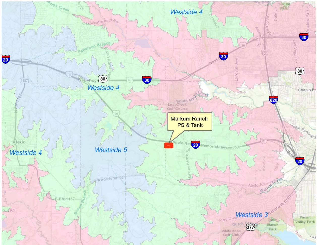
This map shows the location of the Markum Ranch Pump Station and Ground Storage Tank as well as the Westside III pressure plane (in pink), the Westside IV pressure plane (in green) and the Westside V pressure plane (in purple).
