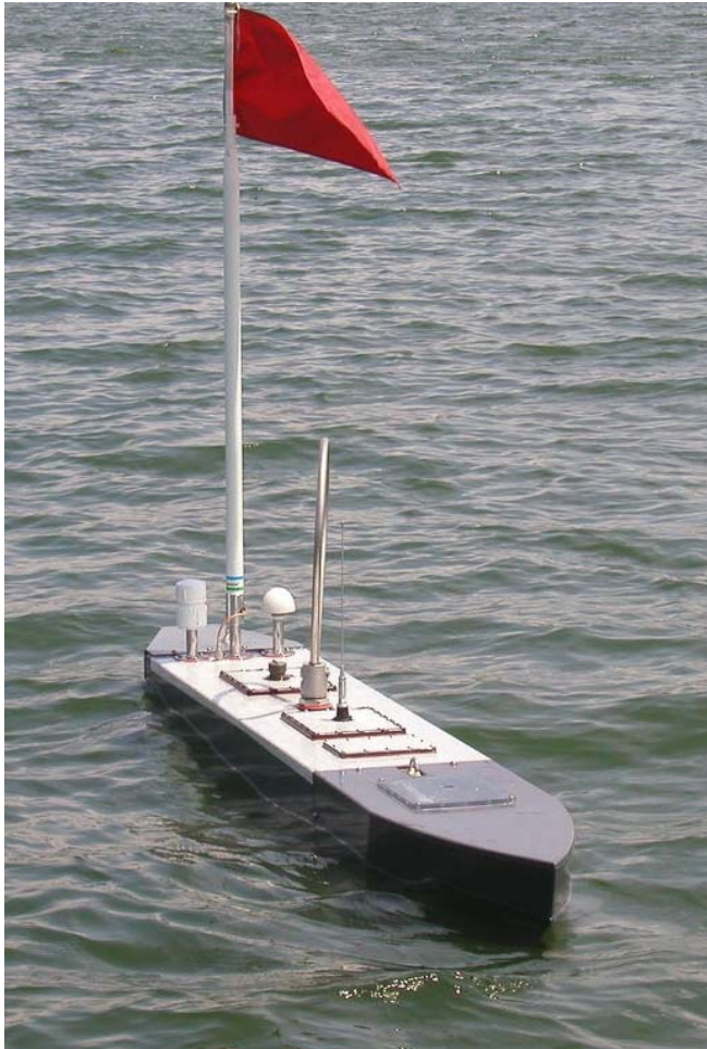
Branch Water Robotic Survey Vehicle
