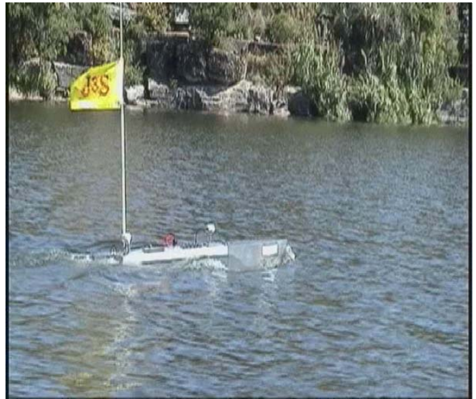
Branch Water Robotic Survey Vehicle
