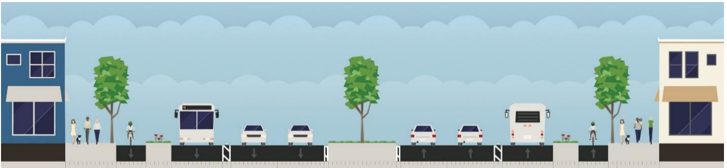
Figure 11: Proposed East Lancaster Ave Cross Section
