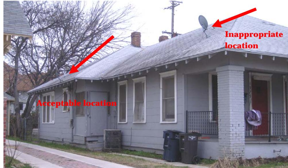
The installation of other roof top mechanical equipment such as air conditioning units and telecommunications equipment is not appropriate and can only be installed in non-visible locations.
