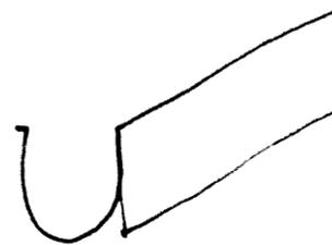
1/2 round gutters are appropriate for all types of eaves, especially where the fascia board is absent.
