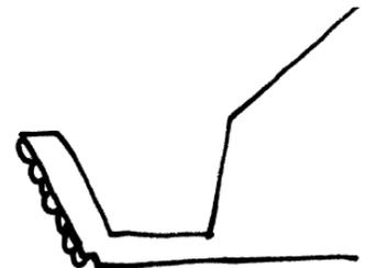
Built-in gutters are appropriate for open eaves and boxed eaves.
