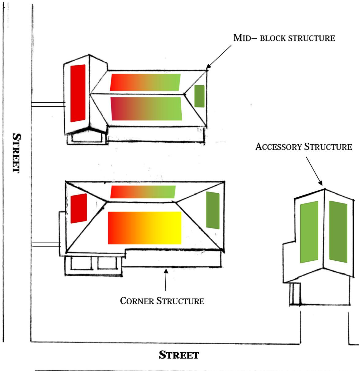
Prior to installing solar technology on-site, try improving the energy efficiency of the structure through other passive methods such as awnings, and screens. When placing solar panels on-site, consider the impact that the technology will have on the historic character and fabric of the site. Consider the following locations prior to requesting the installation of solar technology on historic structures:
