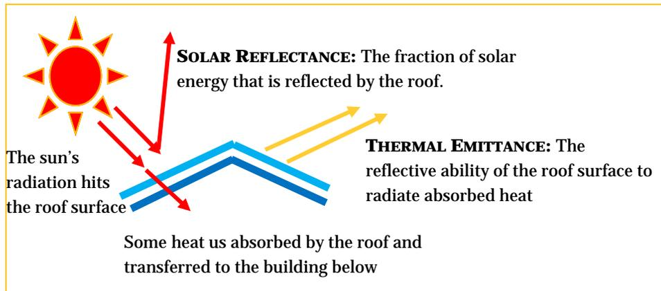
Cool roofs reflect and emit the sun's heat back into the sky instead of transferring it to the structure. Their average energy saving range from 7-10%. There are several different types of cool roofs. They range from coatings for metal roofs and flat roofs to reflective granules on asphalt and other synthetic shingles.
