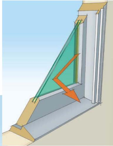
*LEFT: Windows with Low-E coating reflect back part of the summer sun. ABOVE: Windows with Low-E coating reflect back part of room's heat. IMAGE SOURCE: Energy Savers, U.S. Department of Energy.*
