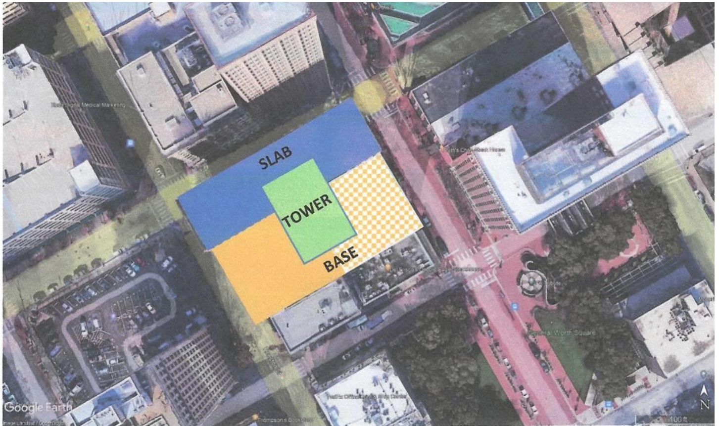
Map 8: Delineation of the three segments of the building: slab, base, and tower. Checkered area of the base indicates the area where a fourth story and a small four-story addition were constructed in 1961. Google Earth Pro image, retrieved October 8, 2021.
