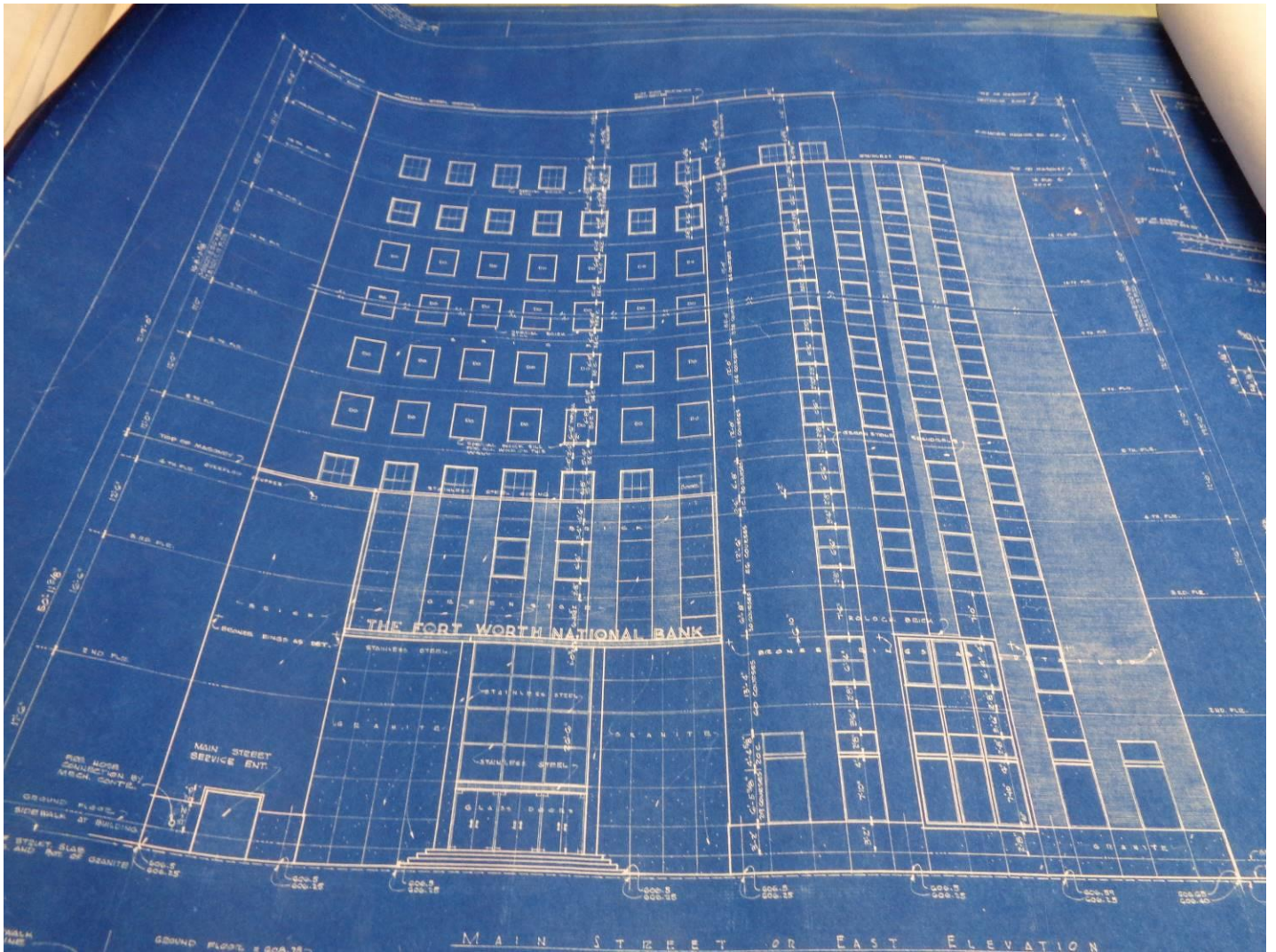
Figure 3: Blueprint, Fort Worth National Bank Building, Preston M. Geren, Architect and Engineer. Main Street (east) elevation (Floors 1-7 and 14-16) before 1961 addition. Plan provided by Benbrooke Electric Partners LLC.
