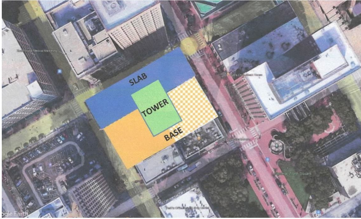
Figure 12 Delineation of the three segments of the building: slab, base, and tower. Checkered area of the base indicates the area where a fourth story and a small four-story addition were constructed in 1961. Google Earth Pro image, retrieved October 8, 2021.
