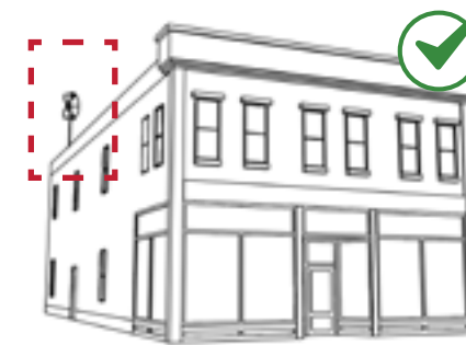
Design the scale and location of a wind turbine to remain subordinate to the historic structure.
