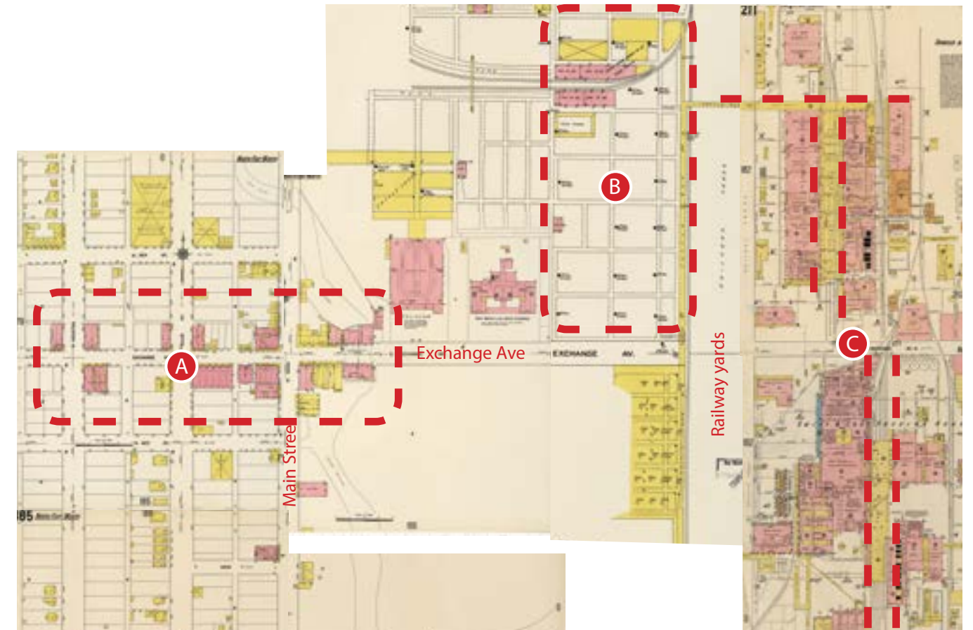
Sanborn Insurance Maps document primary building materials: masonry (including brick and stucco) is shown in red, while frame construction appears in yellow. Metal buildings have a blue color. This 1911 Sanborn map shows a mixture of masonry and wood frame buildings, with only one metal building by the rail yards. Note that no buildings appear for a portion of the area south of Exchange Avenue.
