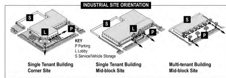
Above: These three diagrams illustrate desirable orientation for industrial corner, mid-block and multi-tenant development sites. Appropriate industrial site orientation for the Industrial Arts Zone.
