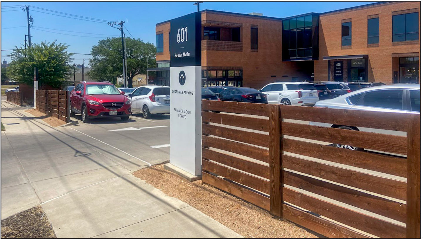
Parking lots that front a street shall be separated from the sidewalk by a decorative and durable screen at least 4 ft. in height.
