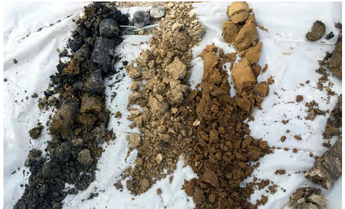
Figure 2-8. Subsurface soil sampling cores are collected at a site to determine environmental impacts, photo by City of Fort Worth.
