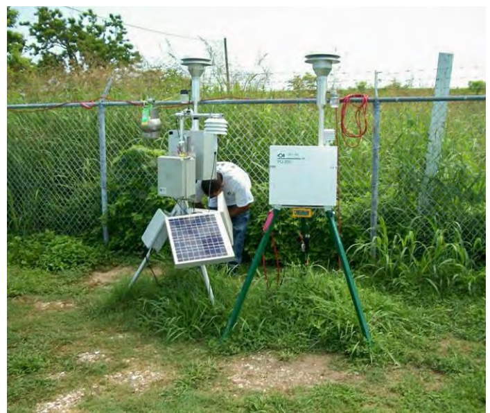
Figure 3-20. The EPA deployed portable air monitors during an oil spill, photo from EPA.
