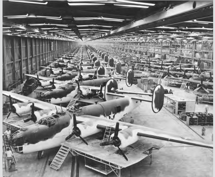
Figure 1-4. B-24 “Liberator” bombers in the Consolidated-Vultee Plant, United States Air Force, 1943. Part of the world's largest double aircraft assembly line in Consolidated-Vultee's Fort Worth plant.
