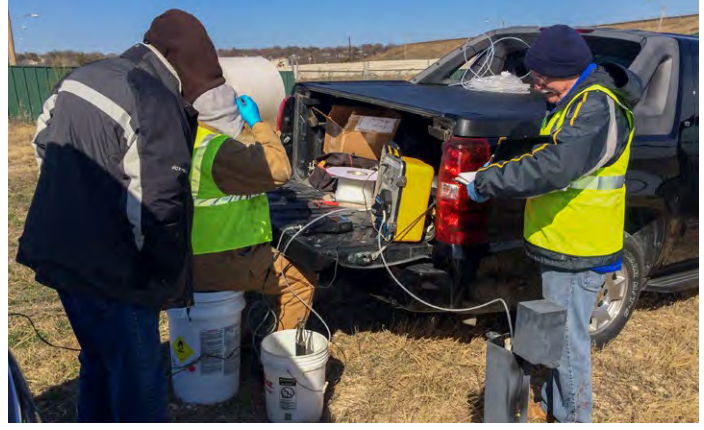
Figure 2-16. Land Quality staff collect groundwater samples from a monitoring well for testing purposes, photo by City of Fort Worth.
