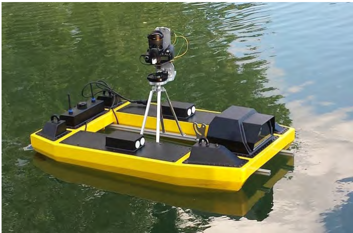
Figure 4-19. A robot deployed on the Gowanus Canal in Brooklyn to collect water quality data, photo from the New York University Polytechnic School of Engineering.
