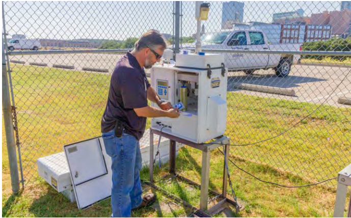
Figure 3-4. An Air Quality Section staff member exchanges a filter on an air sampler.
