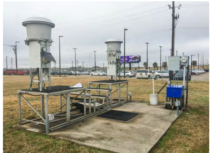
Figure 3-16. PM sampler at a TCEQ monitoring station, photo by City of Fort Worth.
