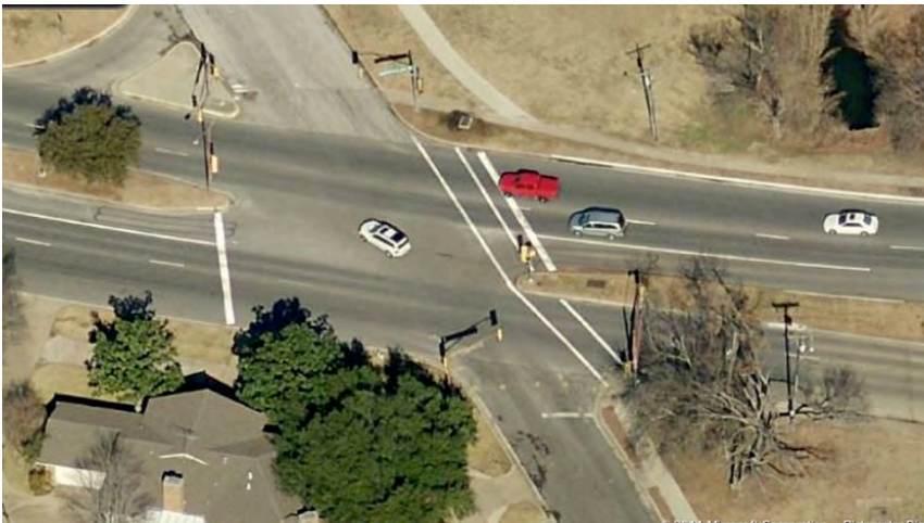
Intersection of Bellaire Dr. S. & Overton Park West * no ADA ramps / median interrupts crossing
