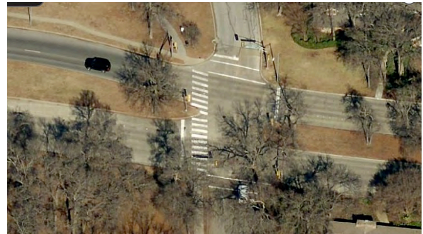
Intersection of Bellaire Dr. S. & Overton Park East * median interrupts crossing / improve transition zone to walks both ends.
