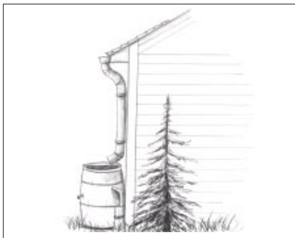
Figure 12. Rooftop Runoff is Collected in a Rain Barrel and Stored for Later Use
