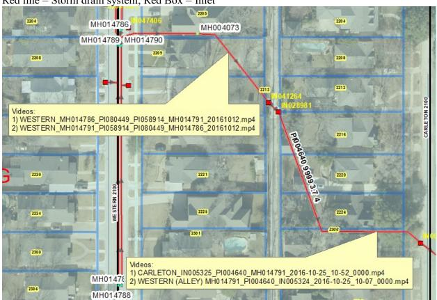
Red line = Storm drain system; Red Box = Inlet
