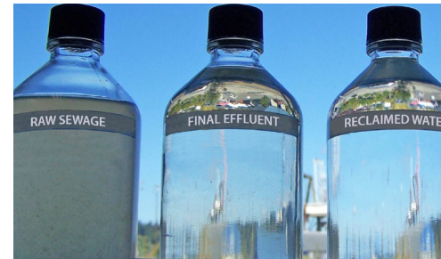
Mary's Creek Water Reclamation Facility site map. Student intern, S. Cisneros, takes part in supervised lab sessions at the Village Creek Water Reclamation Facility. Bottles showing reclaimed water stages.
