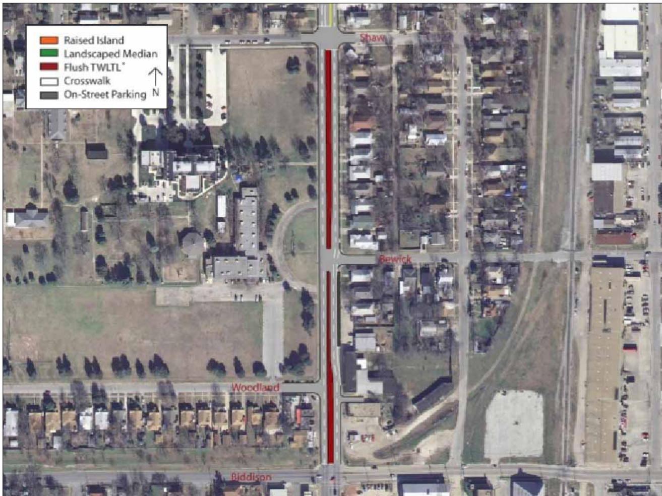
Transportation Concept Detail *TWLTL - Two-Way Left Turn Lane
