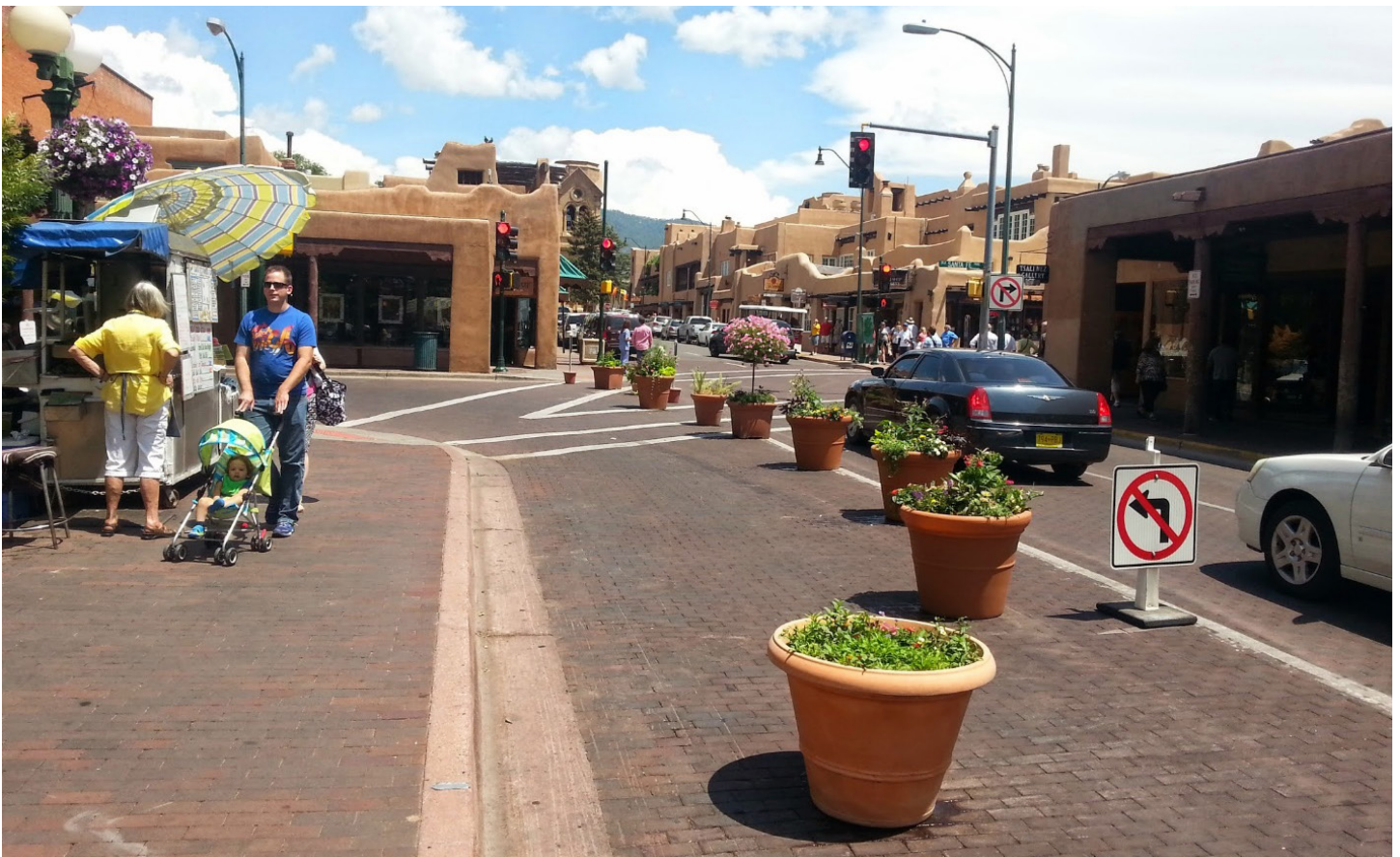
Planters and temporary signage are used to close off a left turn lane and create space for people in Santa Fe, NM in 2014.
