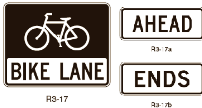
Exhibit 20: Bike Lane Signage
