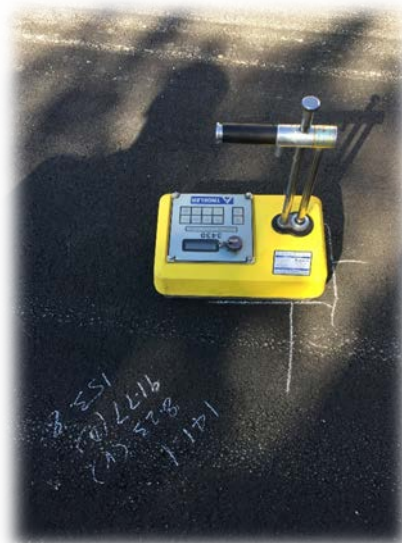
In-place density – Compacted asphalt
