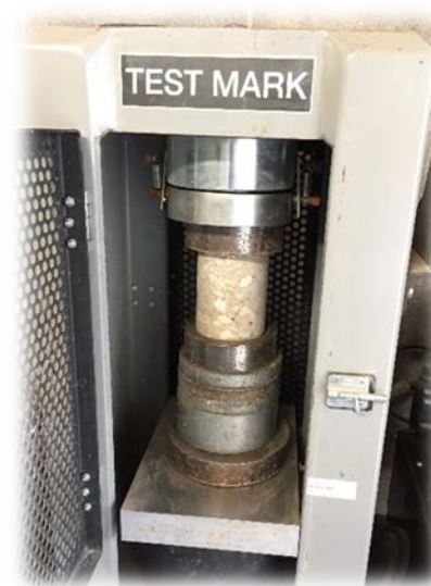
Concrete Strength Test
