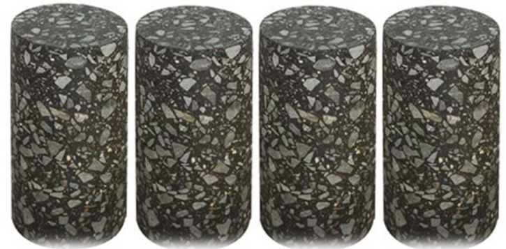
Thickness check – HMAC pavement core
