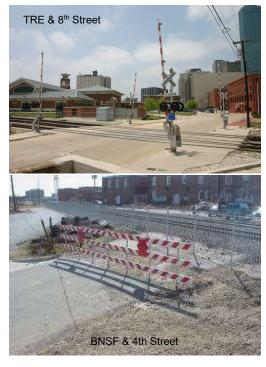
Typical cost range \$10,000 to \$200,000. A closure may entail the installation of one barricade on each side of the track. However, some streets will require a cul-de-sac and right-of-way acquisition, which will increase the cost significantly.
