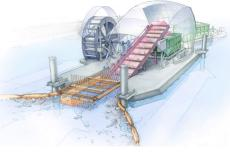
surface using hydropower or solar power, containment booms and a conveyor belt system.
