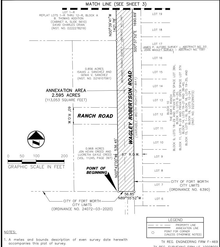
2. Bearing system for this survey is based on the Texas Coordinate System of 1983 (2011 adjustment), North Central Zone 4202.
