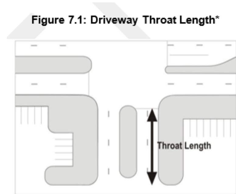
*\*Note: The Fort Worth Traffic Engineering Design Standards and Policy Guidelines document is the source for design details on driveways including widths, radii, angles, slopes, etc.*
