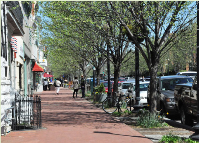
Provide trees and other landscaping as a buffer between autos and pedestrians.
