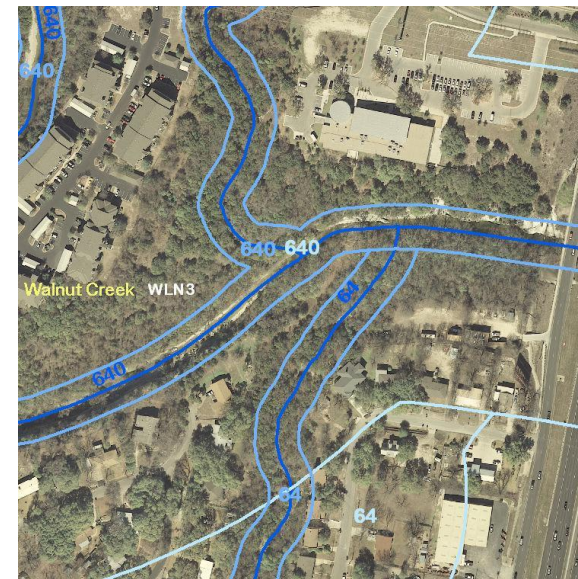
Example of creek line, 50' and 400' buffer base files with respective drainage area threshold values and watershed values labeled for same riparian zone
