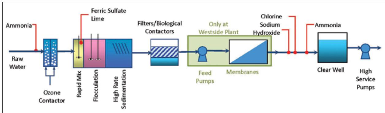
A multi-barrier approach is used in treating drinking water. The treatment process may vary between utilities based on source water quality.
