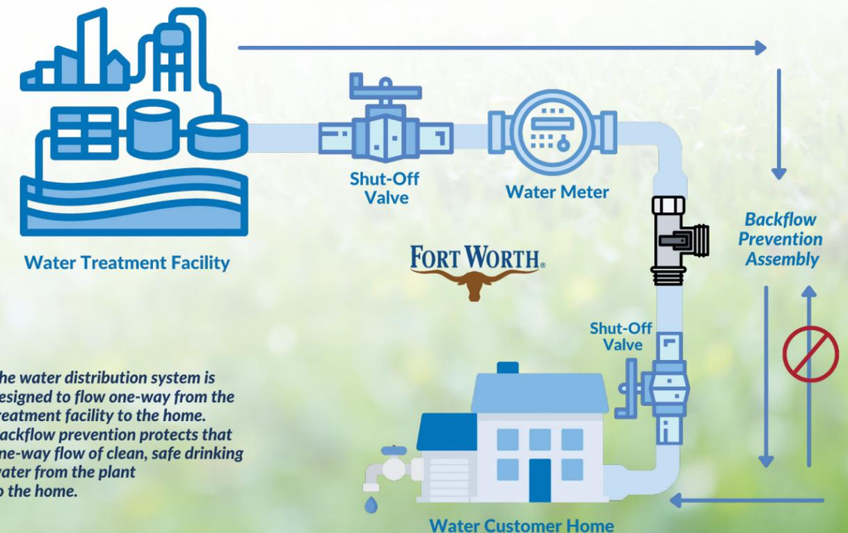
The water distribution system is designed to flow one-way from the treatment facility to the home. Backflow prevention protects that one-way flow of clean, safe drinking water from the plant to the home.
